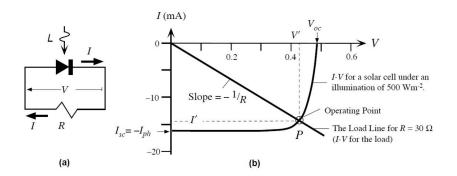
Figure 1: (a) Schematic of a solar cell equivalent circuit. (b) I-V curve under illumination of 500  $Wm^{-2}$ . Adapted from *Principles of Electronic Materials* - S.O. Kasap
